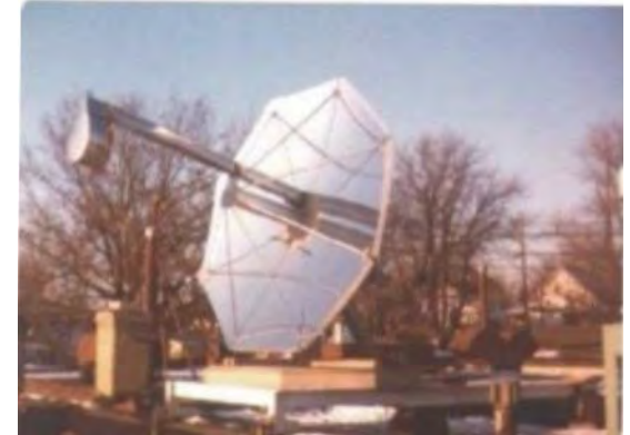
3 M System with Thermal Storage Vault Supplying 900°F Air to a Mass Production Pizza Oven In Elgin, Illinois -1981-
